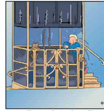
Partially enclosed well with too low enclosure
