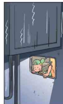
Insufficient safety spaces in headroom and/or pit
