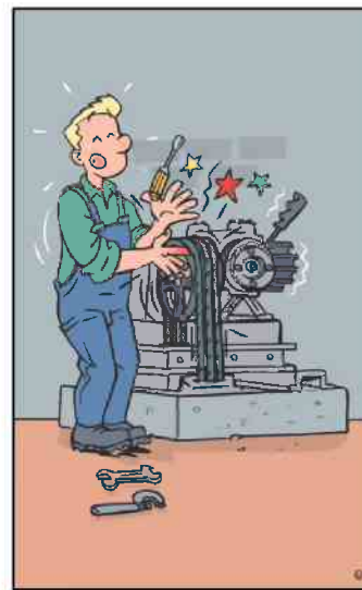
No or inadequate means on sheaves pulleys and sprockets against injury
