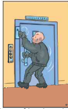
Unlocking of landing door possible without a special tool
