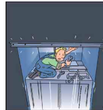
Insufficient safety spaces in headroom and/or pit
